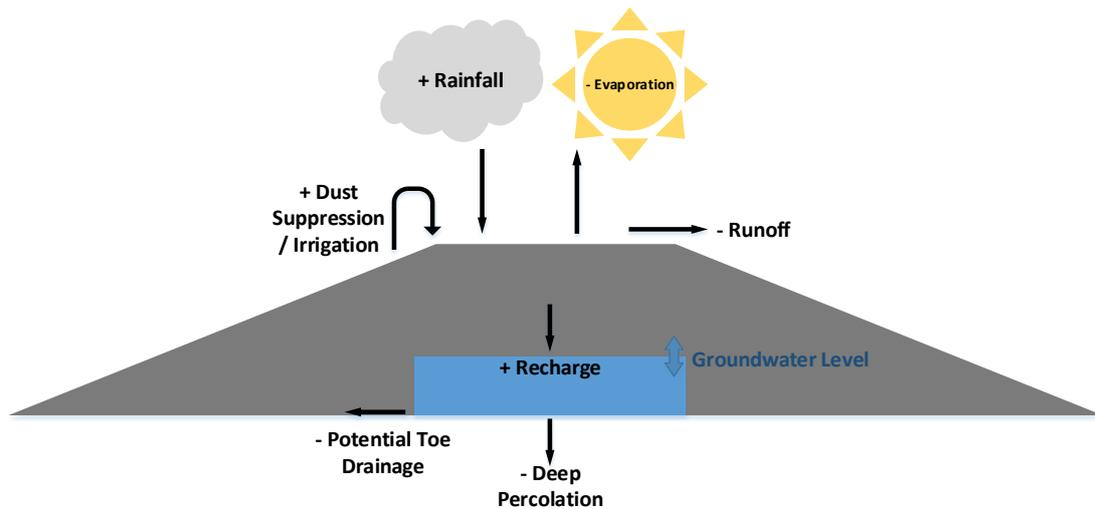
Figure 11.2: Schematic Ash Pile Water Balance
