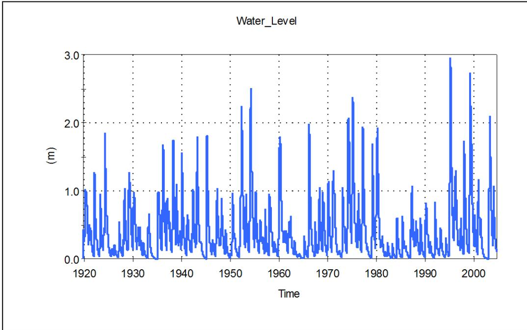
Figure 11.4: Simulated water level in the ash disposal facility
