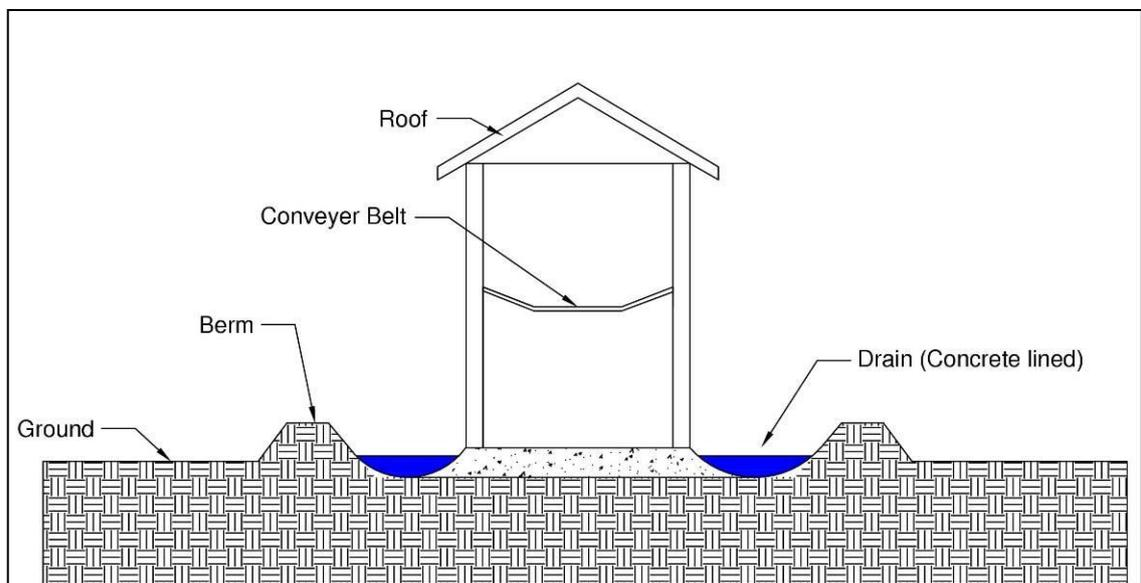
Figure 10.4: Storm Water Measurements for the Conveyor Belt
