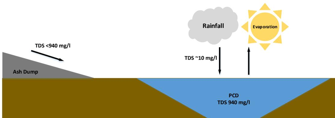
Figure 11.5: Schematic overview of a PCD Salt Balance
