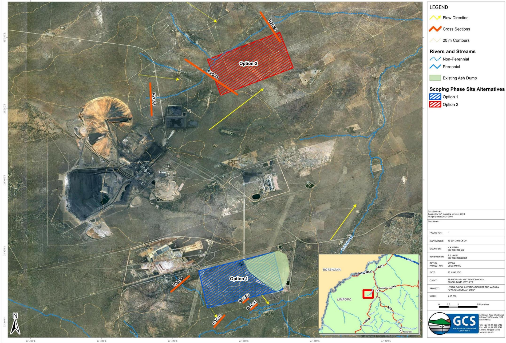
Figure 7.2: Flood line Cross Sections
