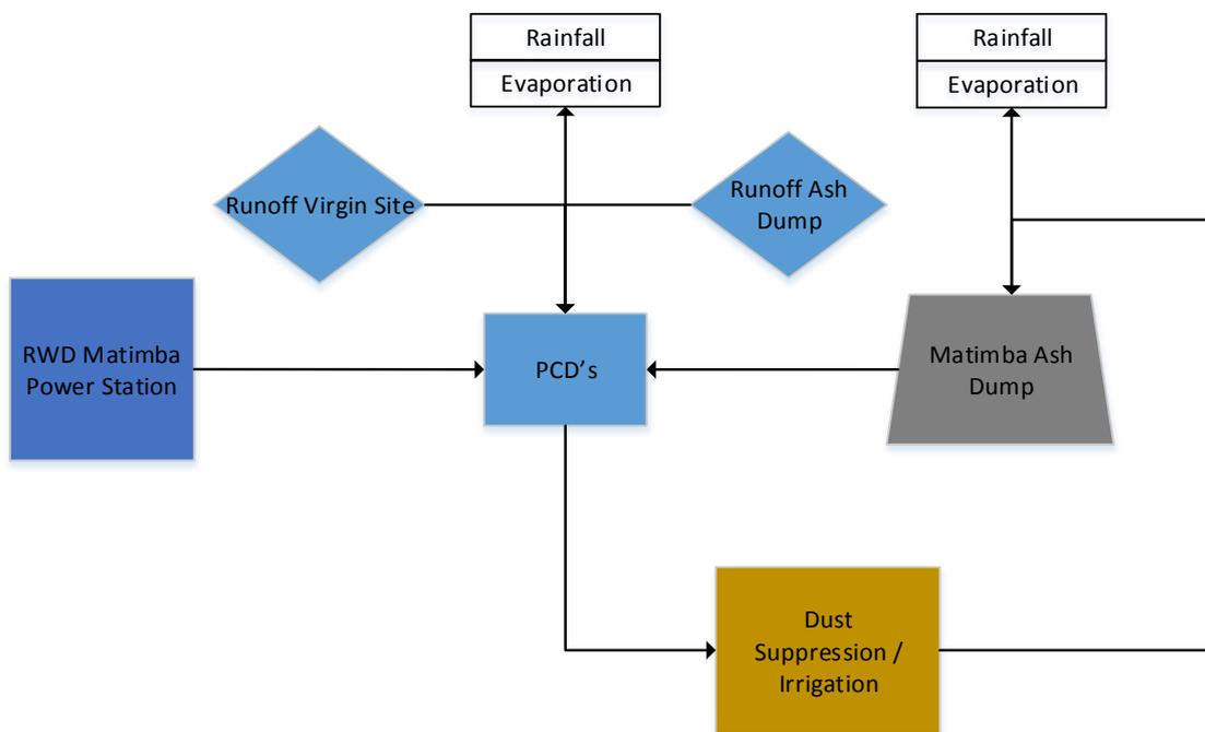
Figure 11.1: Process water flow diagram of the existing Matimba Ash disposal facility
